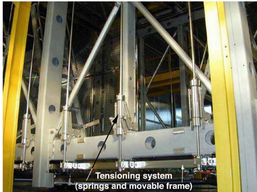
Figure 16. Detail of the wire tensioning mechanics: a 2 m long portion of the wire frame equipped with three tensioning springs.
